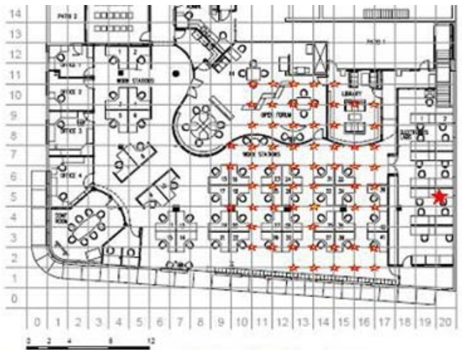
Figure 6. BWRC floor plan with transmitter and receiver locations
