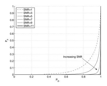
Fig. 3. ROC curves for different SNR values when the rectangular window size is 5, *i.e.* W = 5.
