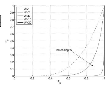
Fig. 2. ROC curves for different rectangular window sizes. The SNR is set to 5dB.
