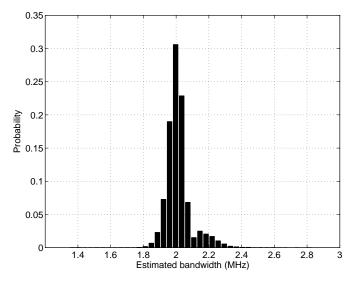
Fig. 4. The histogram of the estimated bandwidth of primary user at 5dB SNR and window size of 5.
