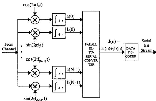
Fig. 2 Receiver section of OFDM modem [2]
