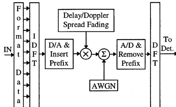
Fig. 3 Block diagram of DFT-based OFDM modem showing channel perturbations simulated
