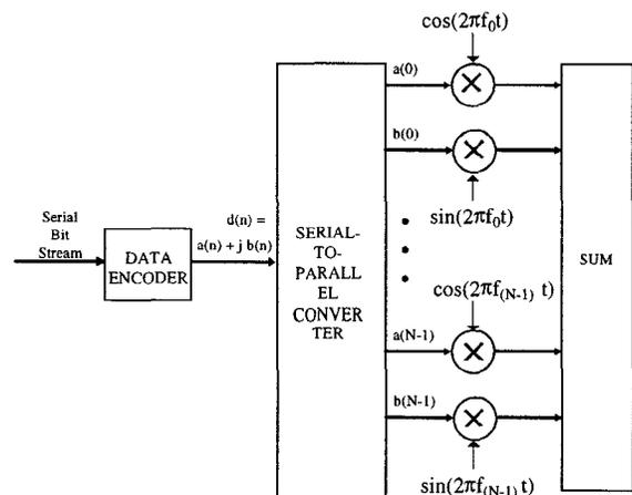
Fig. 1 Transmitter section of OFDM modem [2]
