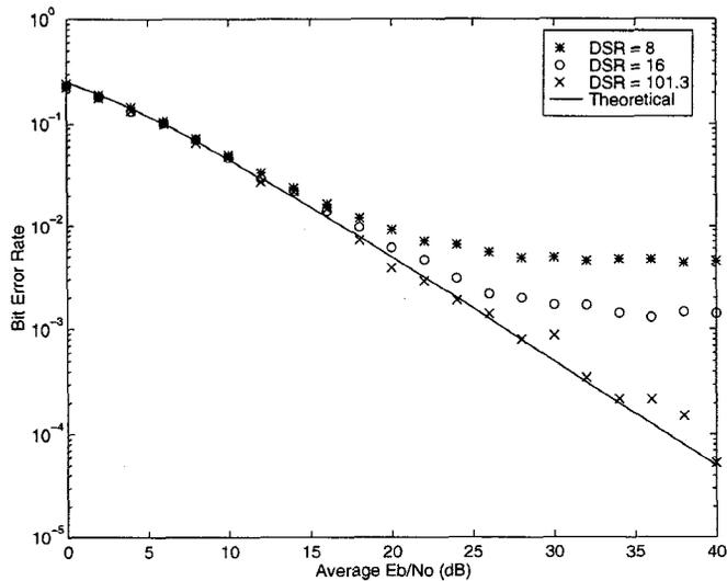
Fig. 4 Performance of 64-carrier OFDM system in Doppler spread Rayleigh fading channel; 4-DPSK
