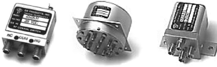
Figure 3.5 Various coaxial switches operating from dc to 26.5 GHz. The switching time is 15 ms. (Reproduced courtesy of DBP Microwave, Pasadena, CA. www.dbp4switches.com )
