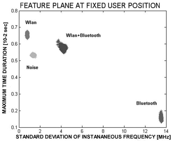
Fig. 8. Feature plane for the four classes at fixed user position.
