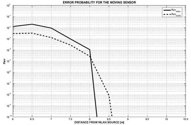
Fig. 18. Error probability of  $\{Noise, WLAN\}$  and  $\{BT, WLAN\}$  classes for the cooperative scenario.
