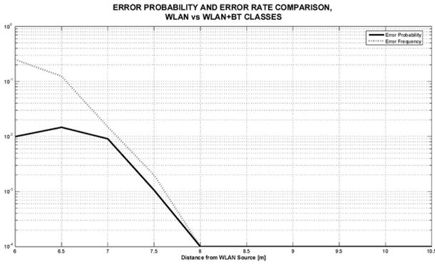
Fig. 20. Error Probability vs Error Rate of  $\{Noise, WLAN\}$  and  $\{BT, WLAN\}$  classes.
