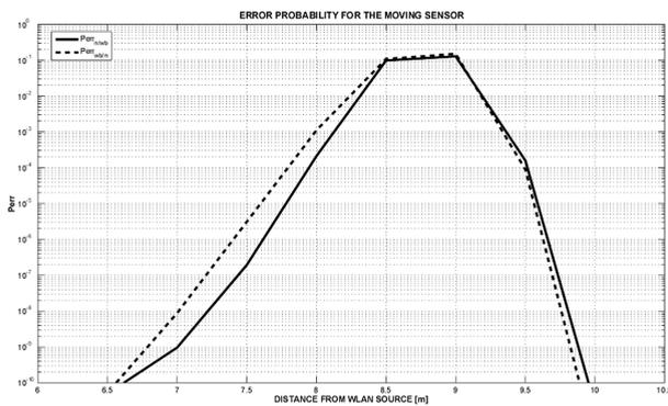
Fig. 17. Error probability of  $\{BT, WLAN\}$  and  $\{Noise, Noise\}$  classes for the stand alone scenario.
