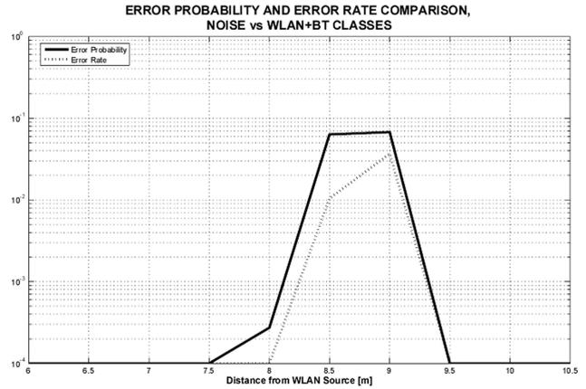
Fig. 21. Error Probability vs Error Rate of  $\{Noise, Noise\}$  and  $\{BT, WLAN\}$  classes.
