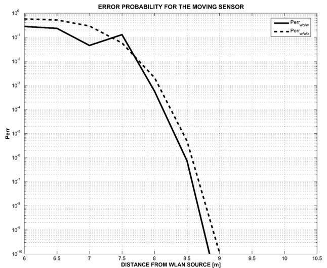
Fig. 19. Error probability of  $\{Noise, WLAN\}$  and  $\{BT, WLAN\}$  classes for the stand alone scenario.
