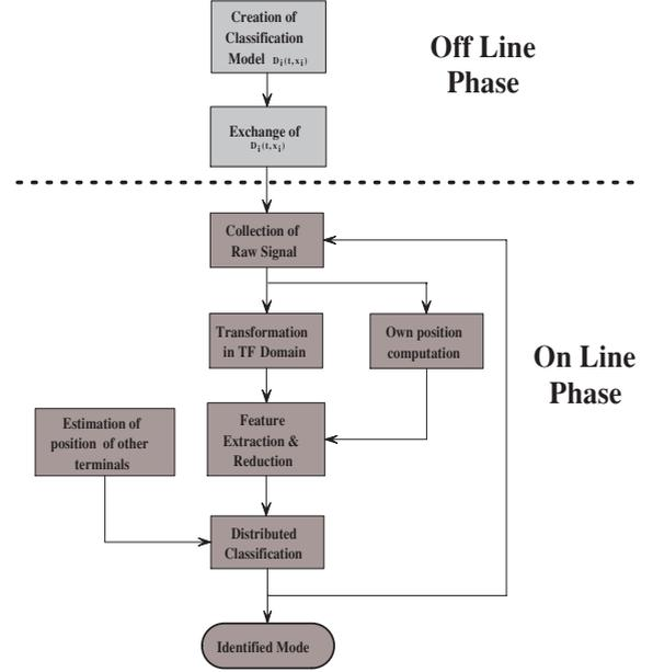
Fig. 15. Flow chart of spectrum sensing algorithm.
