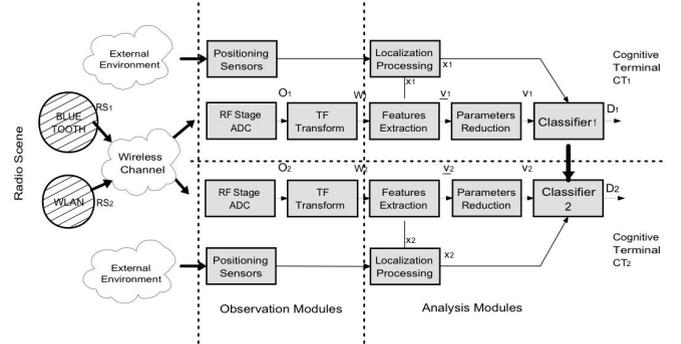
Fig. 7. Logical Architecture of sensing and analysis modules of two Cooperative Terminals.
