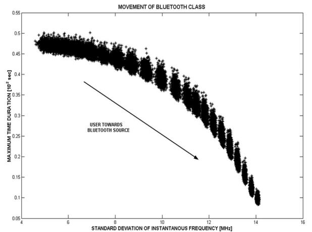
Fig. 9. Feature plane for the Bluetooth class during the movement of user.
