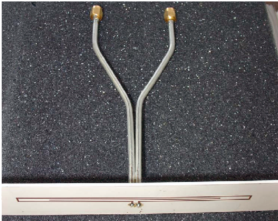
Figure 6.10 Hardware test model of the RPFDA with coaxial feed network.
