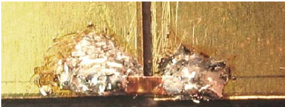
Figure 5.11 Close-up of copper tape RF switch for RPIFA hardware test model.
