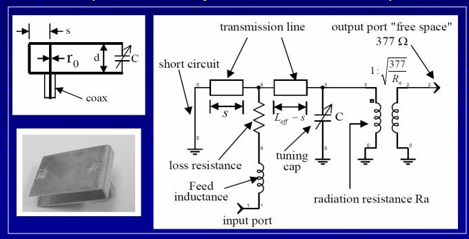
□ In the case that operating frequency should be sweep on a narrow range and on discrete values. SPA is a good choice
