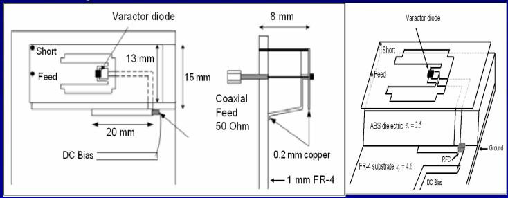
In the case that operating frequency should be change in a relative wide range with continuous values Varactor tunable PIFA can be a good choice.
