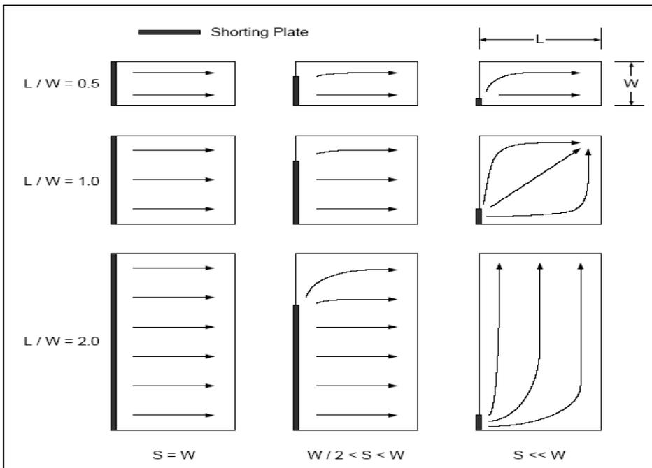
**Figure5.** Surface current on PIFA top plate for various top plate aspect ratios and grounding strap widths.
