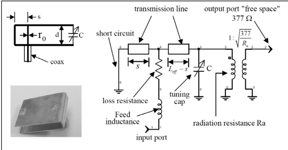
Figure7. SPA antenna and its equivalent circuit
