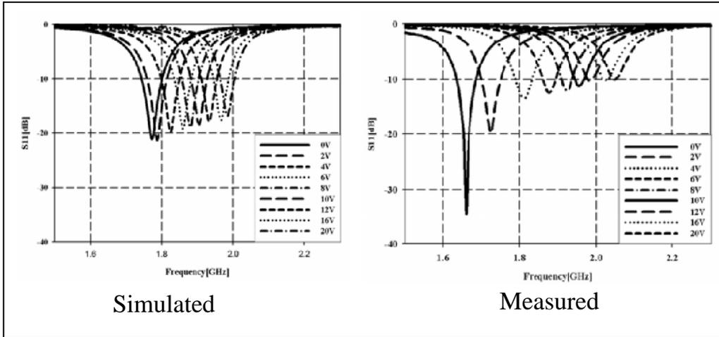
**Figure11.** Varactor tunable PIFA antenna with U-shaped slot results ( $S_{11}$  in dB)
