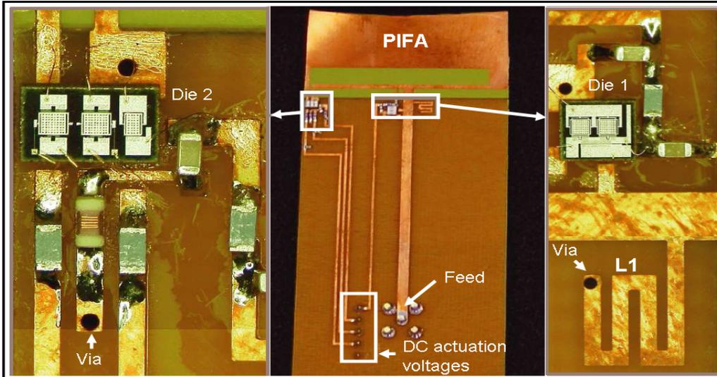
Figure 14. Multi-band MEMS Switched PIFA
