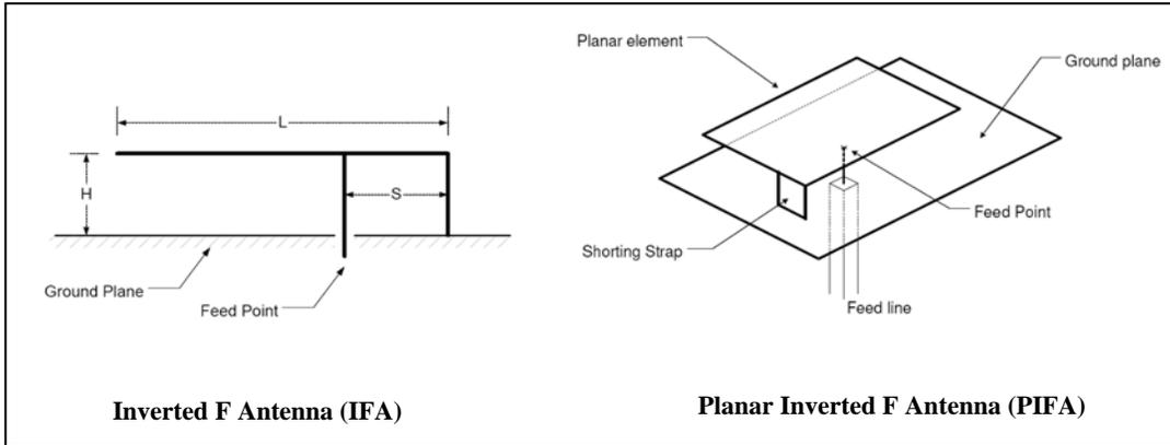
**Figure4.** Inverted F Antenna (IFA) and Planar Inverted F Antenna (PIFA)
