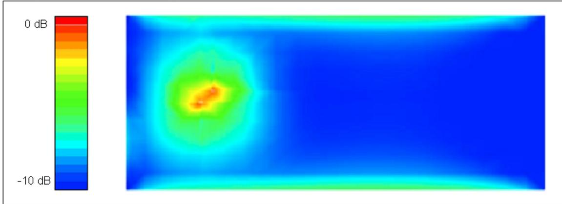
**Figure 6.** Average current distribution on PIFA ground plane computed using IE3D.
