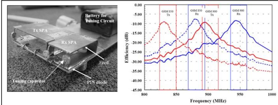
**Figure9.** The SPA antenna hardware and the measurement results
