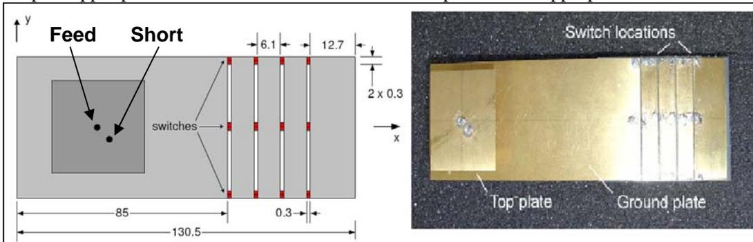
Figure 16. PIFA reconfigurable bandwidth antenna with extendable ground plate
