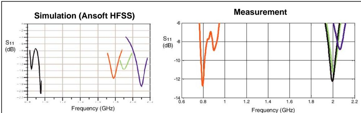
Figure 15. Multi-band MEMS Switched PIFA results
