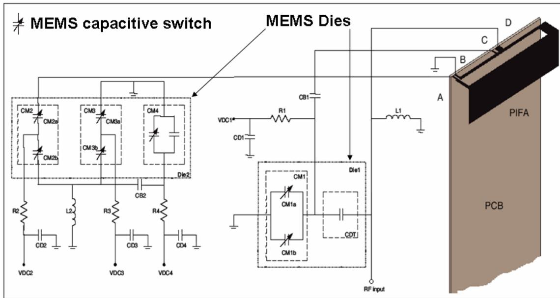
**Figure13.** MEMS switched PIFA and its circuit
