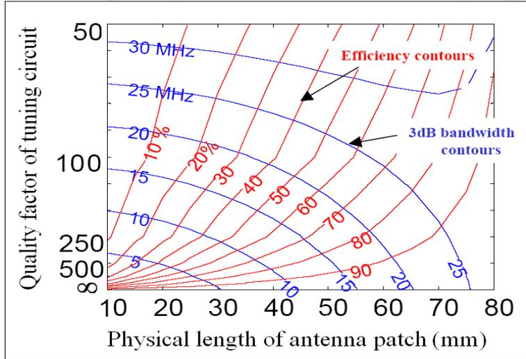
Figure8. The interdependency between bandwidth and efficiency
