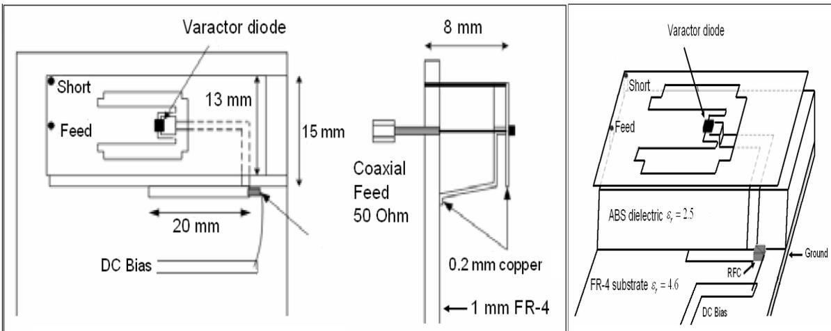
**Figure10.** Varactor tunable PIFA antenna with U-shaped slot structure
