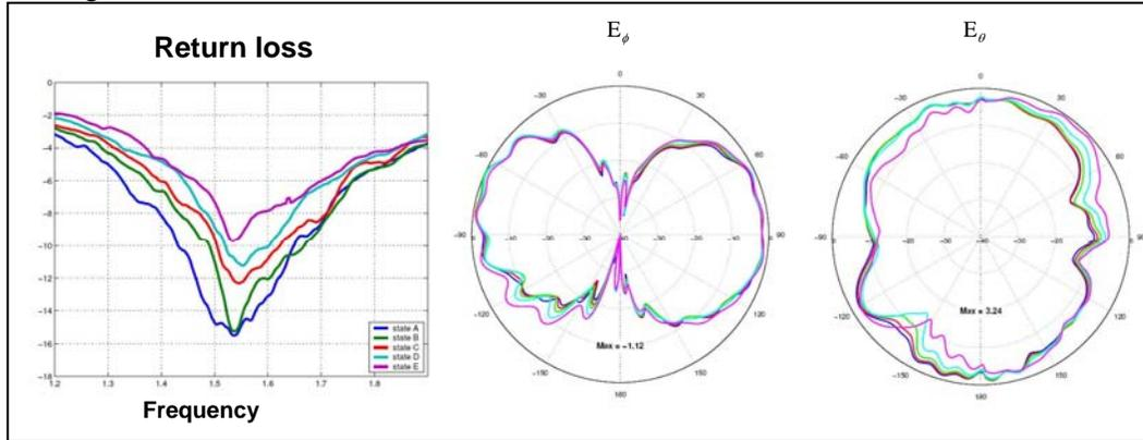
Figure17. PIFA reconfigurable bandwidth antenna, return loss and pattern measurements
