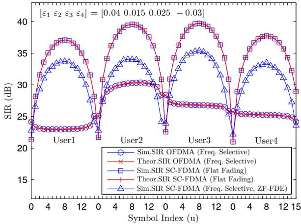
Fig. 6 Received SIR as a function of symbols index in block subcarrier allocation for  $\Upsilon_1$  CFO vector
