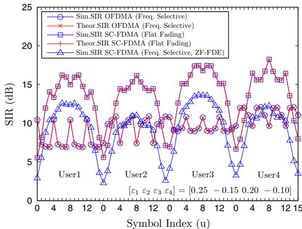
**Fig. 9** Received SIR as a function of symbols index in block-interleaved subcarrier allocation for  $\Upsilon_2$  CFO vector
