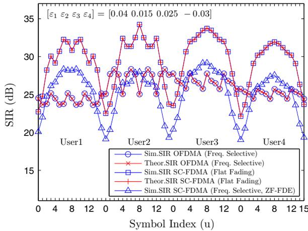
**Fig. 8** Received SIR as a function of symbols index in block-interleaved subcarrier allocation for  $\Upsilon_1$  CFO vector
