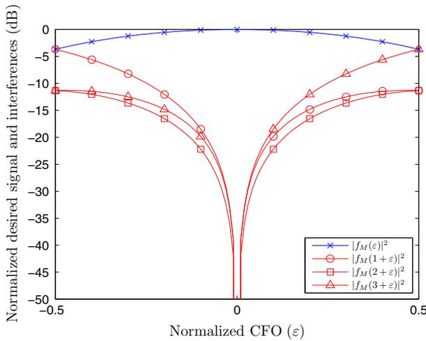
**Fig. 3** The normalized desired signal and MAI powers as functions of normalized CFO for an IFDMA uplink system with  $N = 64$  subcarriers and  $M = 4$  active users
