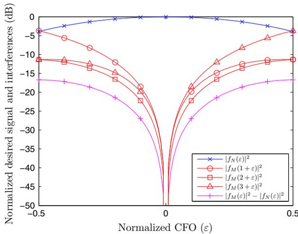
**Fig. 2** The normalized desired signal, ICI, and MAI powers, as functions of normalized CFO for an interleaved OFDMA uplink system with  $N = 64$  subcarriers and  $M = 4$  active users
