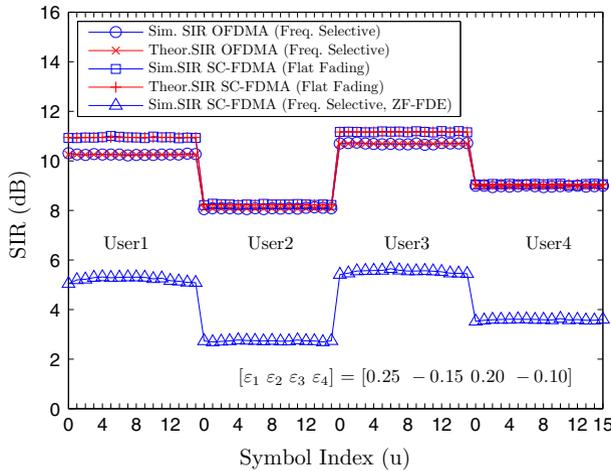
Fig. 5 Received SIR as a function of symbols index in interleaved subcarrier allocation for  $\Upsilon_2$  CFO vector
