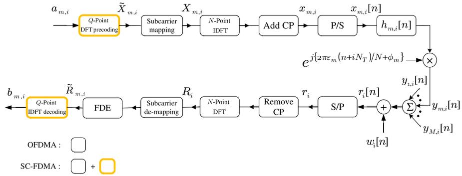
**Fig. 1** The baseband equivalent of OFDMA/SC-FDMA uplink system for the  $i$ th transmitted block in the presence of CFOs
