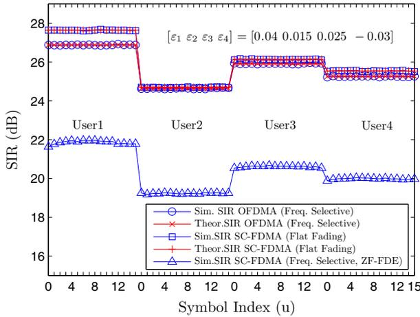
Fig. 4 Received SIR as a function of symbols index in interleaved subcarrier allocation for  $\Upsilon_1$  CFO vector
