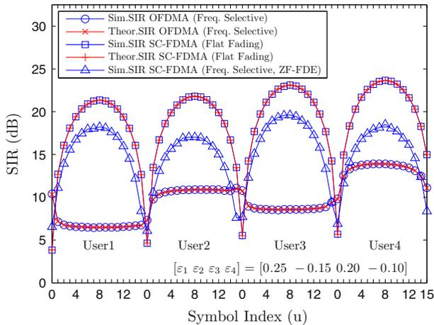
Fig. 7 Received SIR as a function of symbols index in block subcarrier allocation for  $\Upsilon_2$  CFO vector
