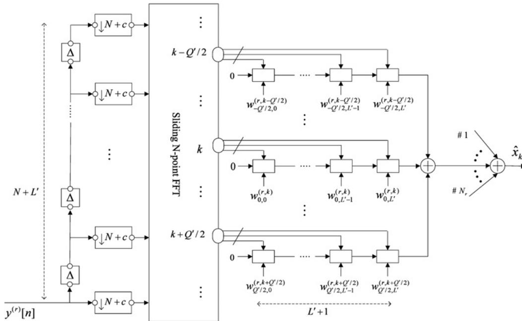
Figure 4 Prop-PTEQ for the  $k$ th subcarrier
