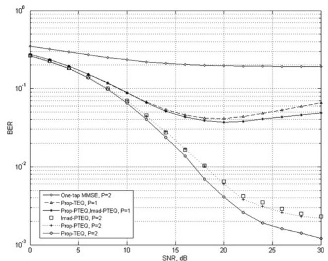
Figure 7 BER comparison for SISO-OFDM system ( $N_r = 1$ )
