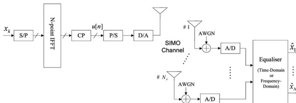
Figure 1 SIMO-OFDM system model
