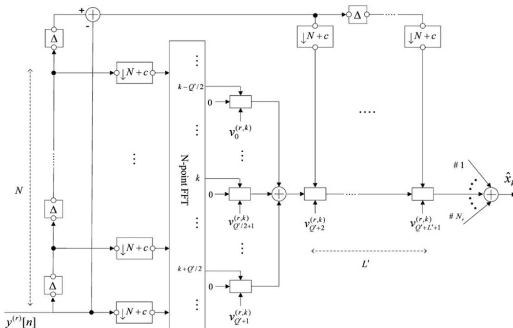
Figure 5 Prop-LC-PTEQ for the  $k$ th subcarrier
