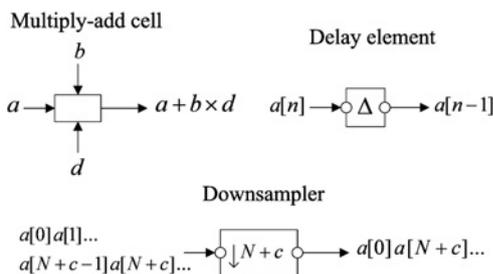
Figure 3 Signal flow graph building blocks
