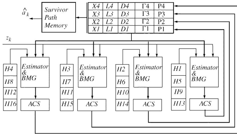
Fig. 8. A parallel architecture for joint data detection and channel estimation (parallel state-computation structure).
