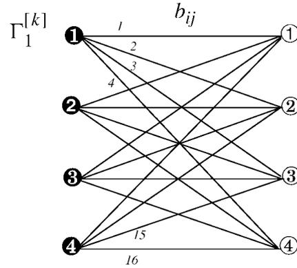
Fig. 7. The trellis diagram for the Viterbi algorithm.
