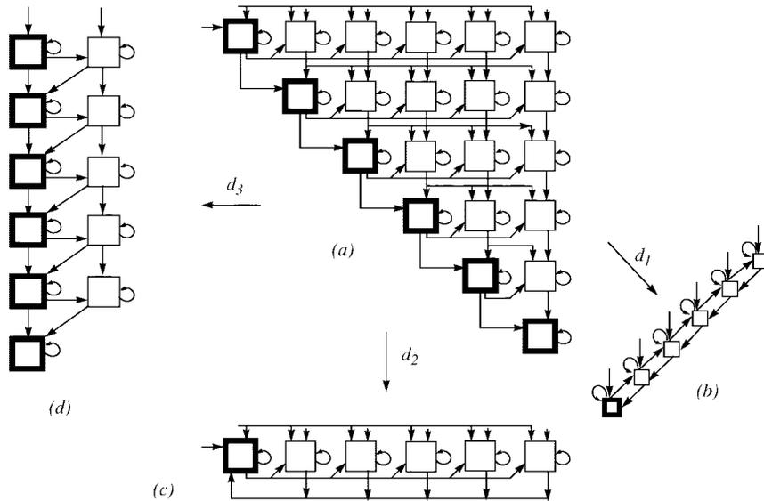
Fig. 5. Mapping the systolic structure of the correction algorithm to a smaller number of processors.
