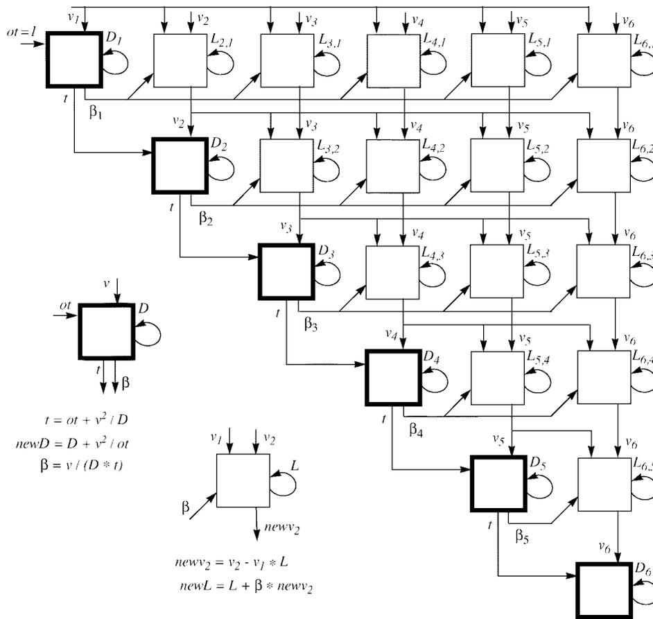
Fig. 4. A systolic VLSI structure for implementation of the LDC algorithm.
