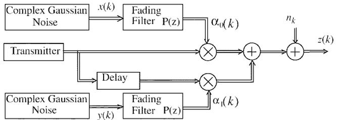
Fig. 2. The fading channel model.
