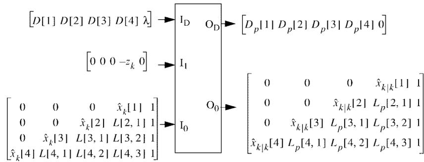
Fig. 3. The data structure for the inputs and outputs of the Jover-Kailath algorithm [3].
