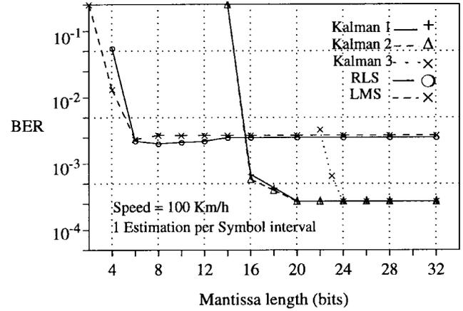
Fig. 11. The effects of changing the wordlength on estimation methods ( $E_b/N_o = 15$  dB). See Fig. 10 for details.
