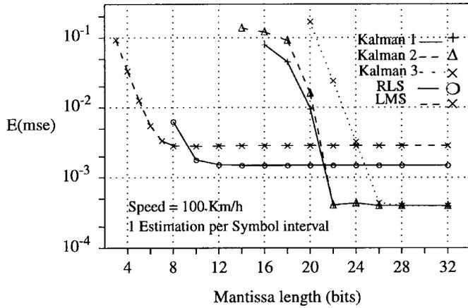
Fig. 10. The effects of changing the wordlength on estimation methods ( $E_b/N_o = 15$  dB). Kalman 1 represents the WGS method, Kalman 2 is for the correction method, and Kalman 3 is the direct method. PSP method is employed for detection.
