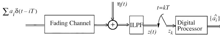
Fig. 1. The signal model for the baseband communication system.
