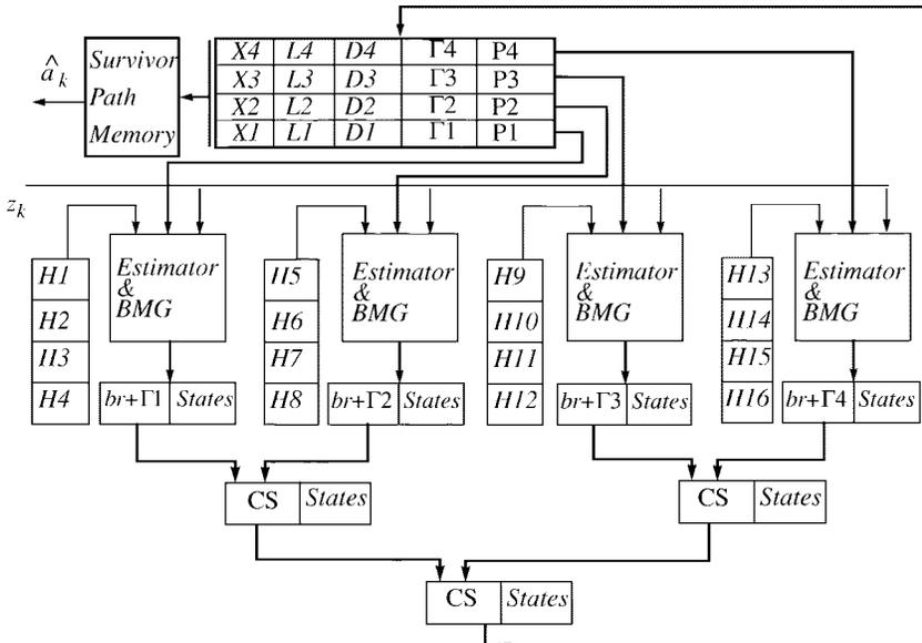
Fig. 9. A parallel architecture for joint data detection and channel estimation (sequential state-computation structure).
