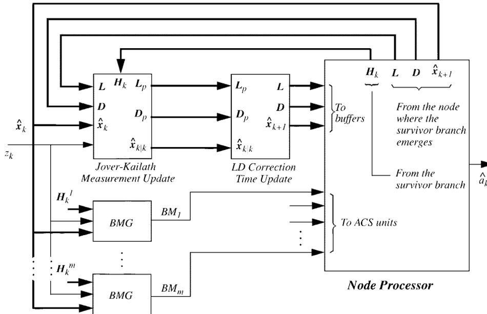
Fig. 6. The required PSP computation for one node (state) of the trellis diagram. First, the branch metrics are generated and the survivor path is found, then the estimator will receive the survivor path information to estimate the channel.
