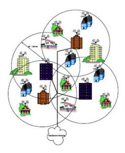
Fig.5. Exemplary 802.22 deployment configuration
