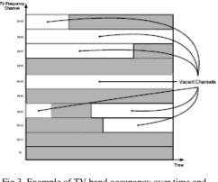
Fig.3. Example of TV band occupancy over time and frequency
