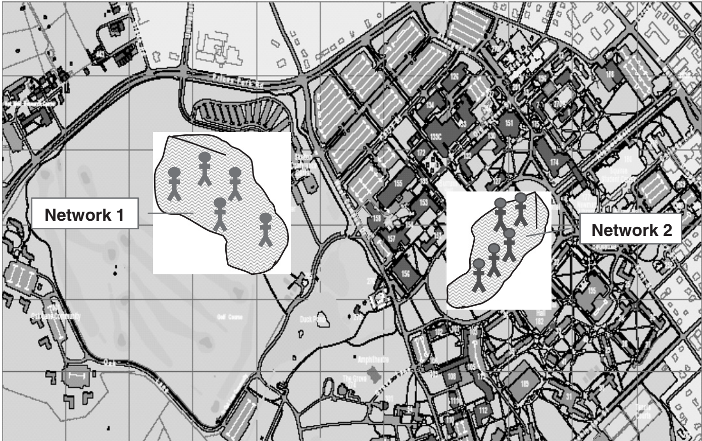
Figure 11.10: DARPA distributed radio scenario. Two ad hoc networks form around two teams of users with intrateam and interteam command requirements, supported by a distributed REM database for both teams.
