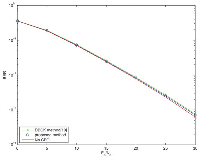
Fig. 3. BER performance for two CFO correction methods
