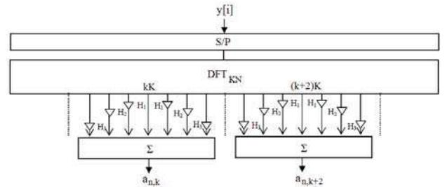
Fig. 2. The in-phase part of a FS-receiver [11]
