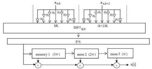
Fig. 1. The in-phase part of a FS-transmitter [11]
