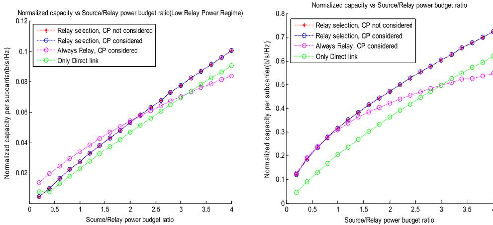
Figure 5. Throughput versus source/relay power budget ratio variation in low (left side) and high (right side) relay power regimes.
