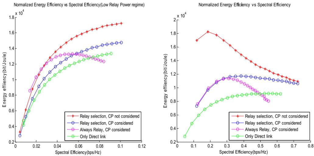
Figure 7. Energy efficiency variation versus spectral efficiency variation in low (left side) and high (right side) relay power regimes.
