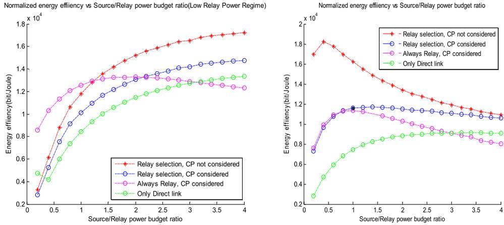
Figure 6. Energy efficiency versus source/relay power budget ratio variation in low (left side) and high (right side) relay power regimes.
