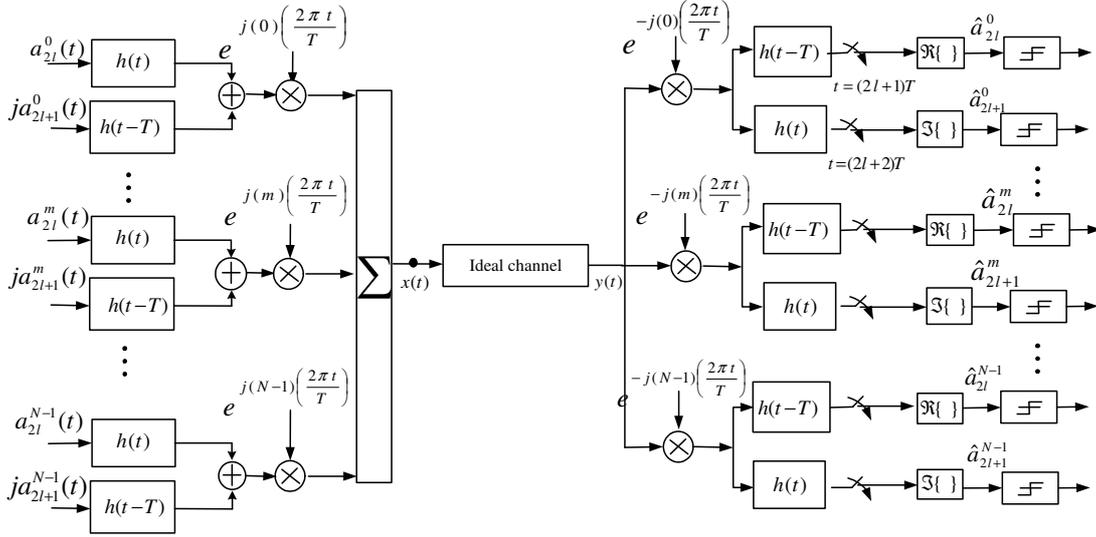
Fig. 1. The baseband representation of OFDM-MSK transceiver (a) Transmitter (b) Receiver
